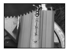
Once the down is in place, measure how long of a flip up you will need. If possible, make it 36-48 inches. Cut it to the needed length.
