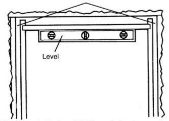
Visually center the top of this frame in the door rough opening. Carefully level the top of the door frame.
